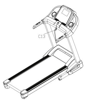
**Step 6:** To check if the running belt runs correctly, placing treadmill in folding position and tightening all the bolts. Then set speed under 3km/h and see if running belt runs without problem.
