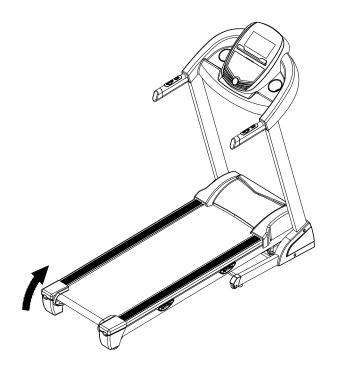
Lift up the machine and force to pull up until you heard "click" that made by safety casing stuck the neumatic c linder.
