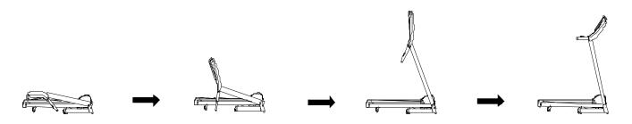
**STEP 3:** According to the picture, tighten the bottom frame with bolt M8\*45(D16) and inner washer(D17). Then locked the console frame with M8\*15 (D13) and inner washer (D17).
