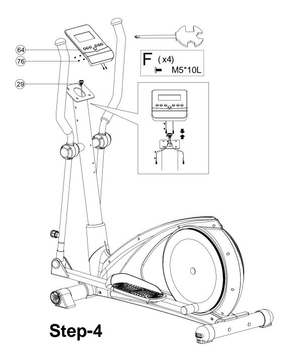
1) Connect the upper computer cable (29) with the computer (64), then fix the computer (64) on the handlebar post (10) by using the screws (76).
