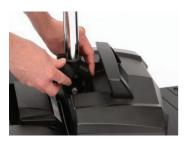
2. Turn the handle to release the battery pack, then lift out the battery pack from the main body of the scooter.
