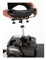
5. Replace the seat and rotate it until it locks in to its correct position.
