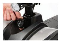
2. Unlock front tiller by pulling the locking knob out and turning 90°.
